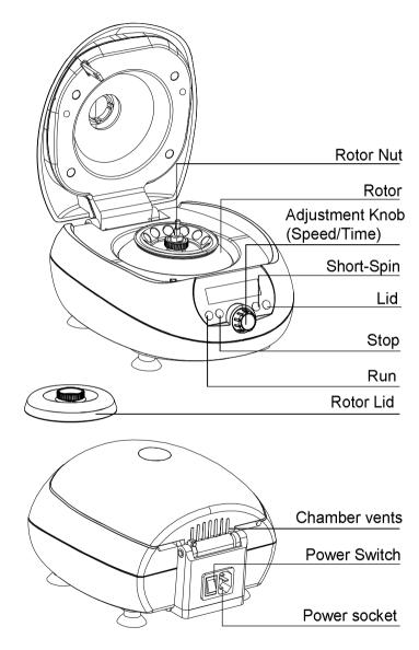
4.4.3 Press "Run" to begin the cycle . Press "Stop" to end the run prematurely. (The remaining run time appears in the display.)
